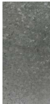
Figure 3 Dull Gray Passivated Zinc
