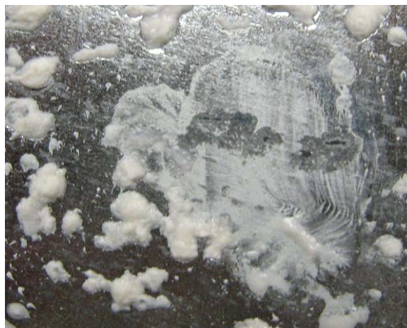
Figure 1 – Waxy White Rust Cells
